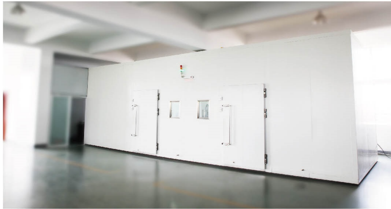
National Standard Enthalpy Testing Room
